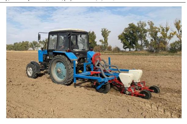
**Figure 1** – Mock-up sample of a combined unit for pre-sowing tillage and sowing seeds FS-1,4 in operation
