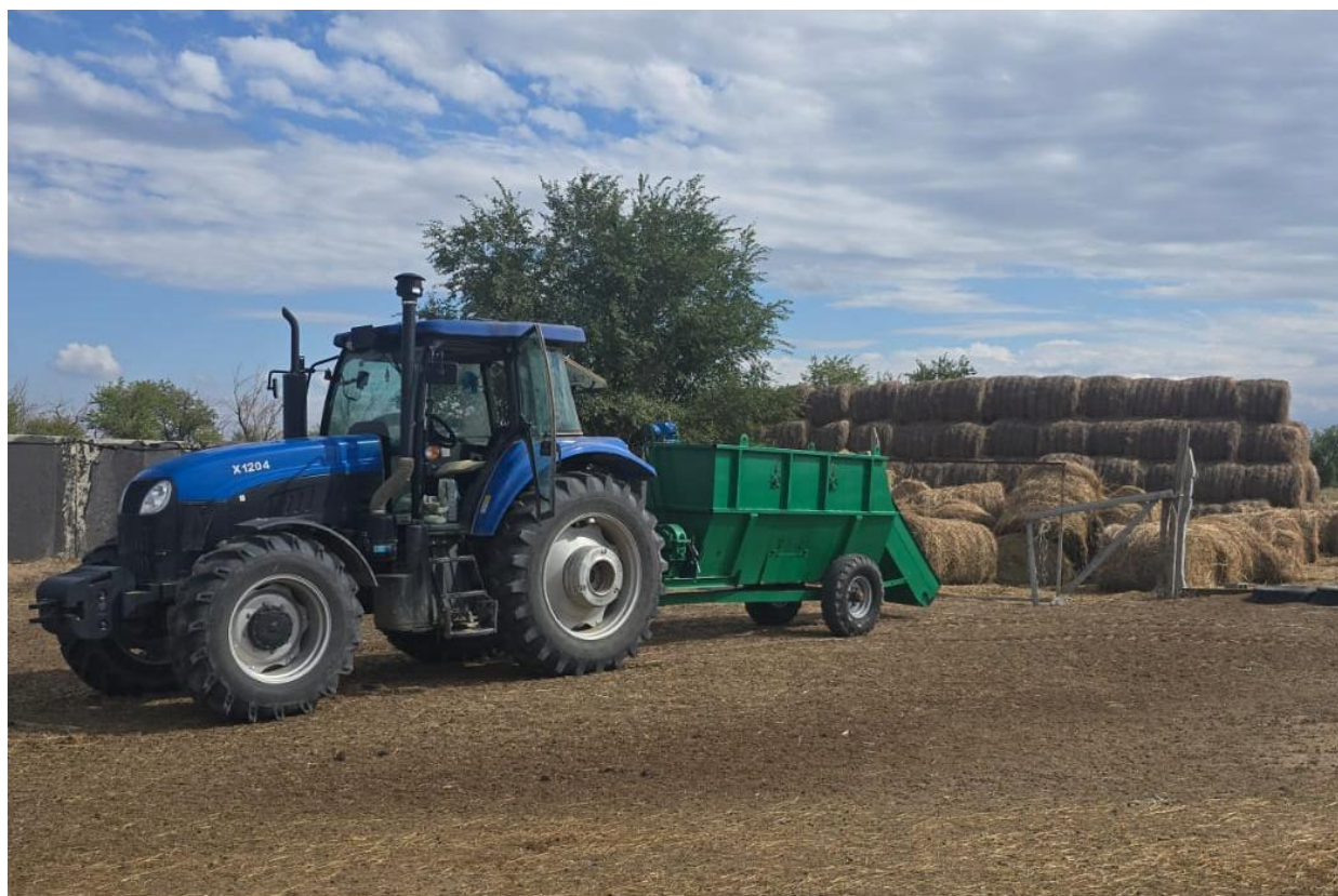
Figure 2 – Field testing of the mini-feed dispenser-mixer attached to a tractor
