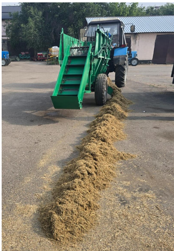
Figure 1 – Laboratory testing of the mini-feed dispenser-mixer for uniform feed distribution
